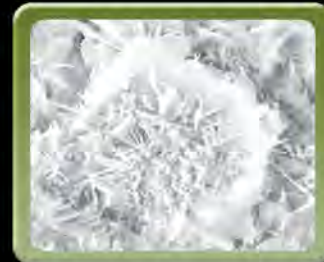
Crystalline structure of OsteoVationEX® after setting
